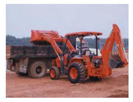
Kubota's performance matched loaders are unrivaled for power and productivity. Increased frame durability, 3,560 pounds of breakout force, 2,200 pounds of lift capacity and a 9'6" lift height are just a few of the impressive features all controlled by a single lever mounted on the operator's right side. The L39's front loader ensures superior overall operation to let you handle your jobs with ease.
