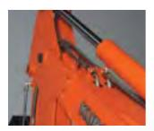
**Enclosed Hydraulics** All hydraulic hoses are routed through the boom and arm for improved hose protection and durability, not to mention excellent visibility and an overall cleaner backhoe design.
