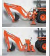
Quick-Mount Attach/Detach Featuring a four-point mount, quick attach system, the backhoe can be removed and installed easily.
