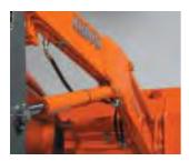
**Protected pipes** The hydraulic pipes are routed through the L39's loader boom for clearer operator views, as well as increased pipe protection and durability.
