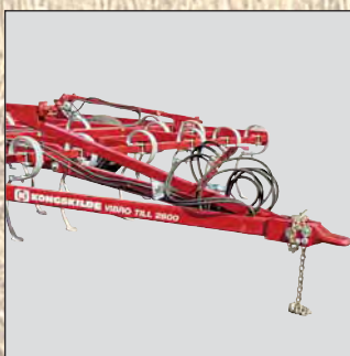
The long drawbar makes turning easy.
