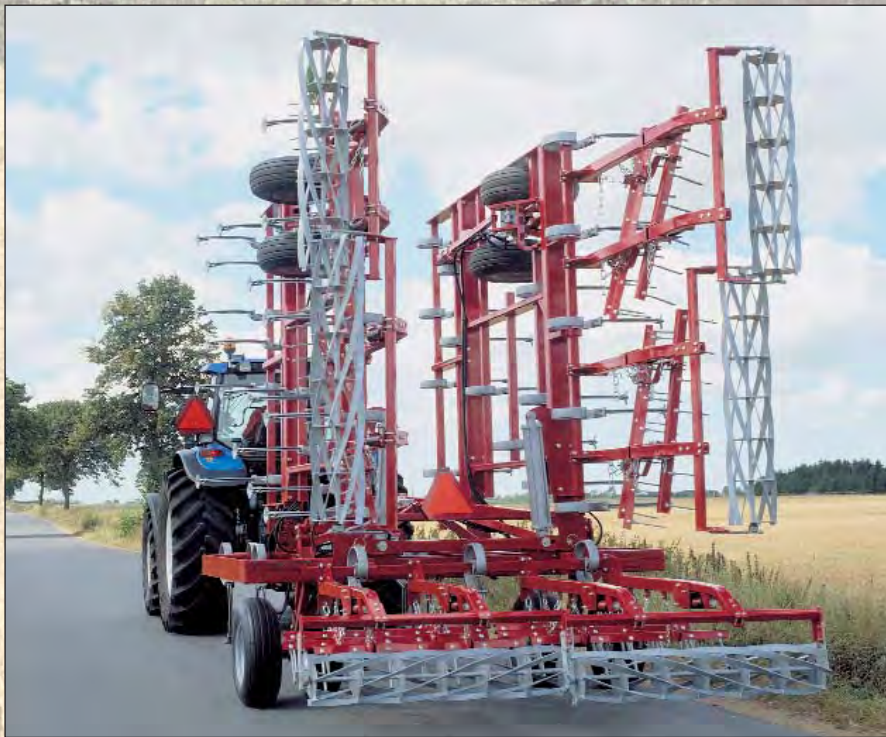
Wings fold hydraulically to a narrow transport width of approx. 3.4 m. The overcentre, locked position assures stability and safe transport.
