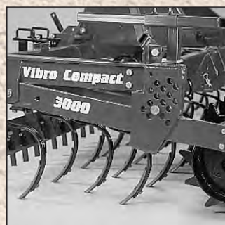
Depth adjustment with pin/hole system.
