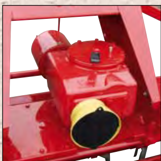
3-speed leverchange gearbox with rear PTO.
