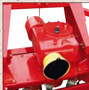
3-speed leverchange gearbox with rear PTO.
