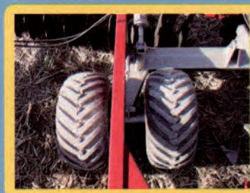
Pneus 400 x 60 x 15,5 Dual tyres 400x60x15,5 (low pressure) Llantas 400x60x15,5
