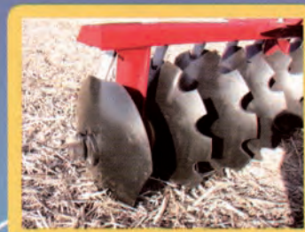
Disco de acabamento Disc blade for finishing Disco borrasurco
