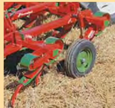
The pneumatic or metal depth wheels are set using screw adjusters and graduated scale allows for precise depth control.
