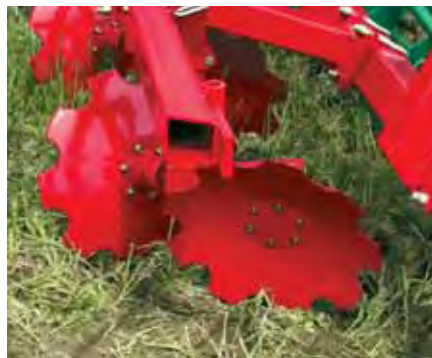
The notched levelling discs are mounted on taper roller bearings. They are height adjustable by pin or screw and are staggered to avoid blockages.
