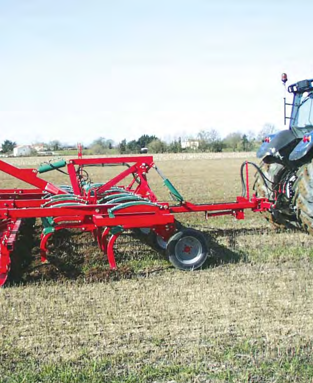
"Auto-reset" tines with Kverneland leaf spring safety protection for use in stony/hard conditions.
