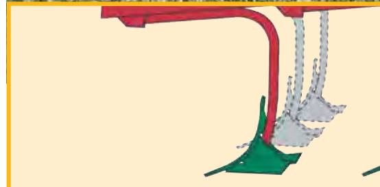
Zone 1: 2 rows of tines Full width cutting over the entire working width Loosening Mixing
